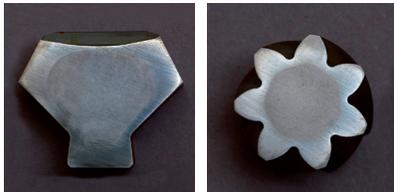
Bishop can also manufacture inductors to supply the customer with a variety of specific heat treatment patterns.
